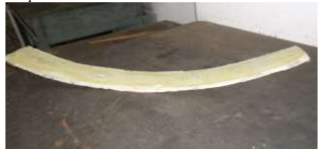
Figure 3: Trimmed final prototype of E-glass/Epoxy composite leaf spring [7]
