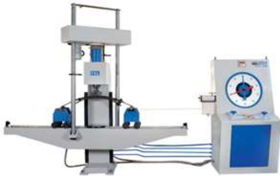
Figure 5: Typical Fatigue Life Testing SPM.
